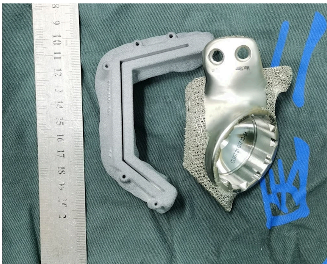
Fig a. A customized 3D-printed acetabular implant features osteointegrable surfaces to enhance bone ingrowth.
