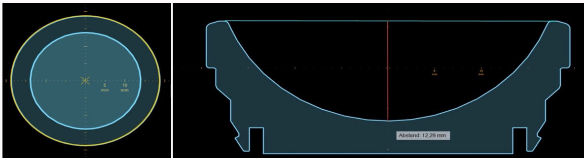
Fig. 2 Screenshot of a measurement on mediCAD 3D shoulder. Left: axial view; the liner is positioned strictly parallel to the axial plane; the centre of the liners' concavity is determined by using a best-fit circle. Right: frontal view; first a tangential line is drawn on top of the concavity (blue line). Then, the jump height is determined by drawing an orthogonal line (red) from the middle to the bottom of the concavity.
