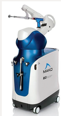
Fig. 1a Stryker Mako robot with hip reamer attachment.
