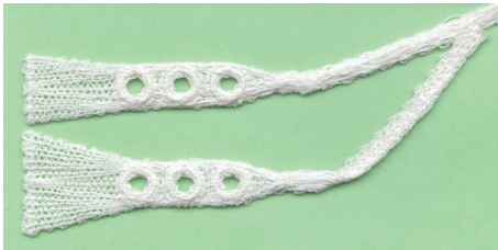
Fig. 14 Nottingham Augmentation Device developed with Julian Ellis (Ellis Developments Ltd 2001)
