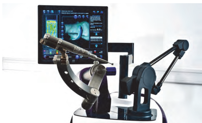
Fig. 1. The Stanmore Sculptor Robotic Guidance Arm, which assists with bone preparation for the implantation of patient-specific implants.
