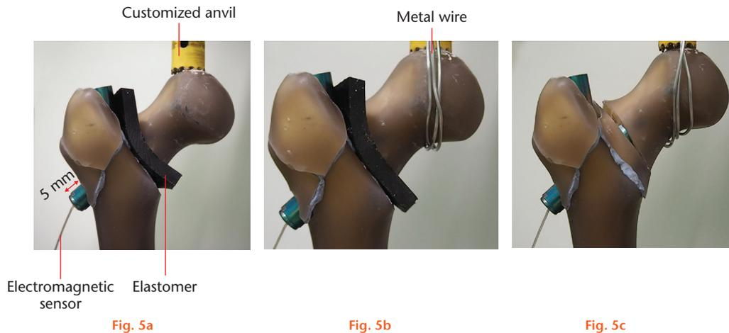
a) Group 1 with unidirectional loading and elastomer; b) group 2 with bidirectional loading with elastomer; c) group 3 with bidirectional loading without elastomer.
