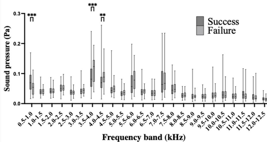
**Fig. 2** The sound pressure (Pa) in different frequency bands (kHz) of successful and unsuccessful press-fit fixation.
